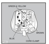
The wire coloured green and yellow must be connected to the terminal marked with the letter  $\langle E \rangle$  or by the earth symbol  $\downarrow$  or coloured green and yellow.
